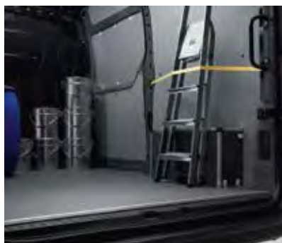
6 mm polypropylene side walls and non-slip floor
