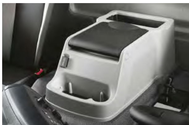
CENTRAL STORAGE COMPARTMENT capacity 15 l, writing surface, bottle holder, cupholder and supplementary 24 V power supply.
