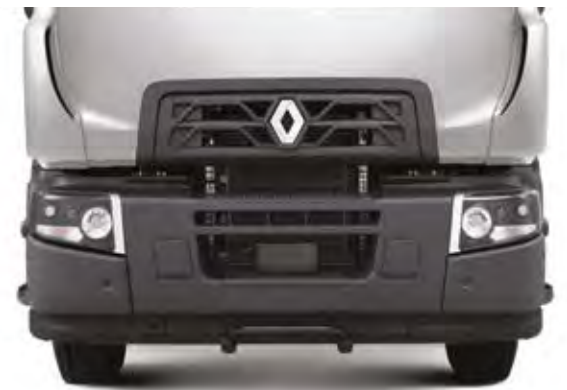
BUMPER WITH STEEL CORNERS (D WIDE) for greater resilience.
