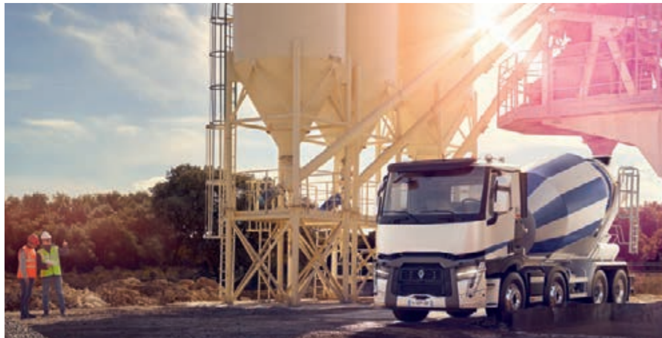
The C XLOAD 8x4 straight truck mixer with an unladen weight of 9 200 kg.
